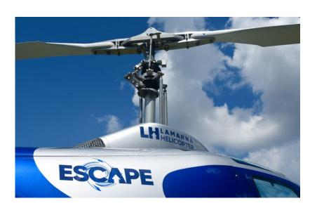
High-efficiency, aerodynamically optimized blades with an infinite lifespan, combined with an elastomeric pitch change hinge, ensure superior-class autorotation.
