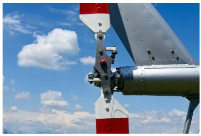
Aluminum alloy blades without ball bearings or flapping hinges keep the tail rotor perfectly centered, reducing vibration levels and maintenance requirements.
